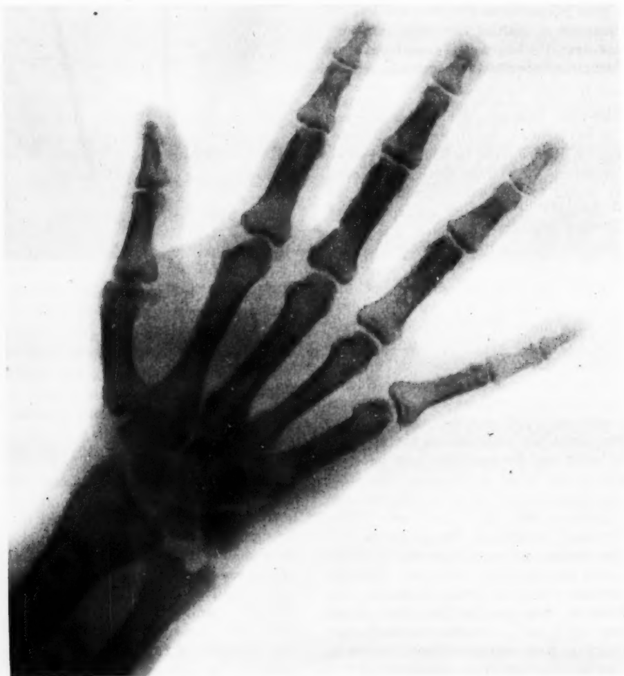
Fig. II-15 Radiograph of a hand made with a 1000-curie \text{Pm}^{147} source at 16 in. Time, 5 sec. Film, Polaroid 3000 X.
